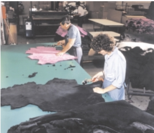
Most waste produced in tanneries is represented by scraps from the actual skins and hides
