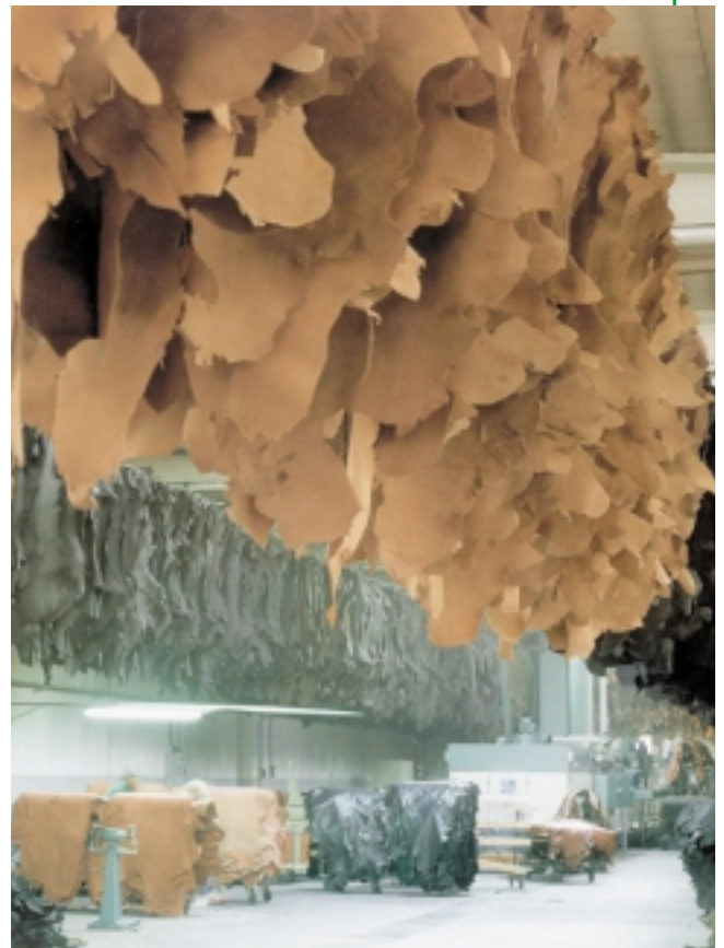
"Overhead chain": traditional method for drying skins
